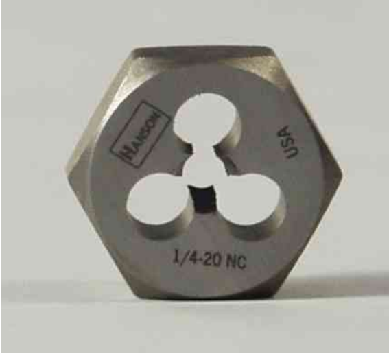
Front of Die (Note taper of threads into hole in center)
