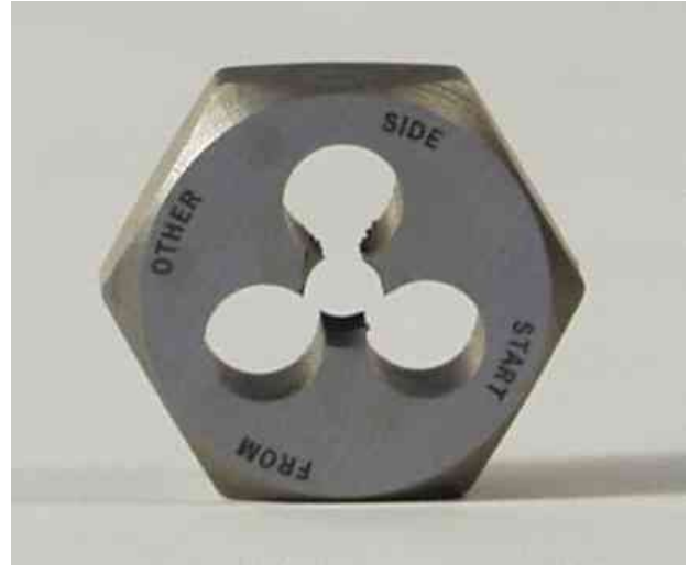
Back of Die (Note lack of thread taper)
