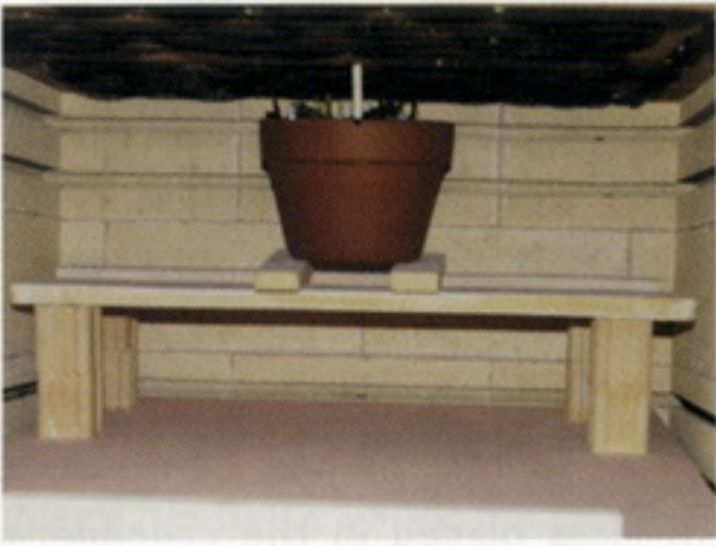
Slant the crucible, or the shelf holding the crucible, for a different effect.
