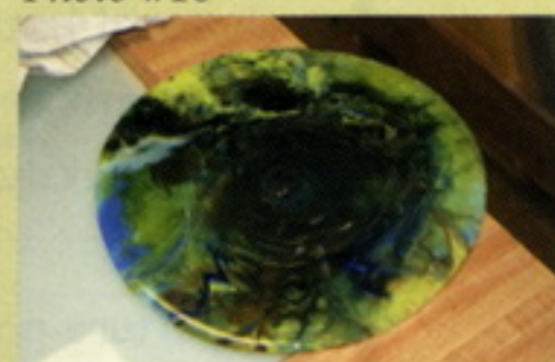
Result of the melt that had been disturbed by the stainless steel fork.
