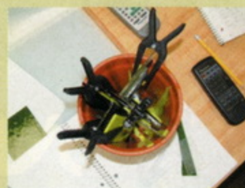
Photo #2 Spring clamps are helpful for loading glass into the pot in a controlled manner, but remember to remove them before firing.
