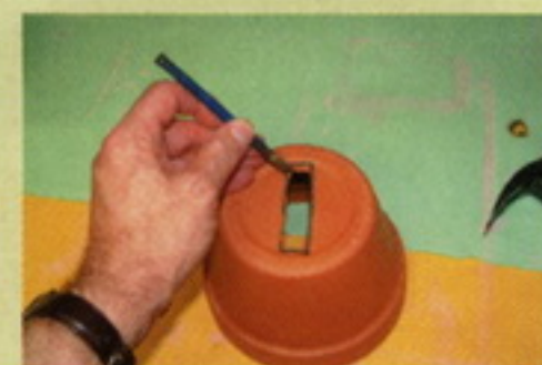
Photo #3 Making a rectangular opening with a hammer and chisel.
